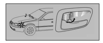
c. The tail and marker lights flash 1 time, the buzzer chirps 1 time, and the doors lock and unlock 1 time. \*
